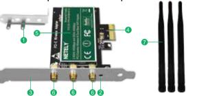
4 PCIE X1 interface 5 Shield cover 6 SMA connector
